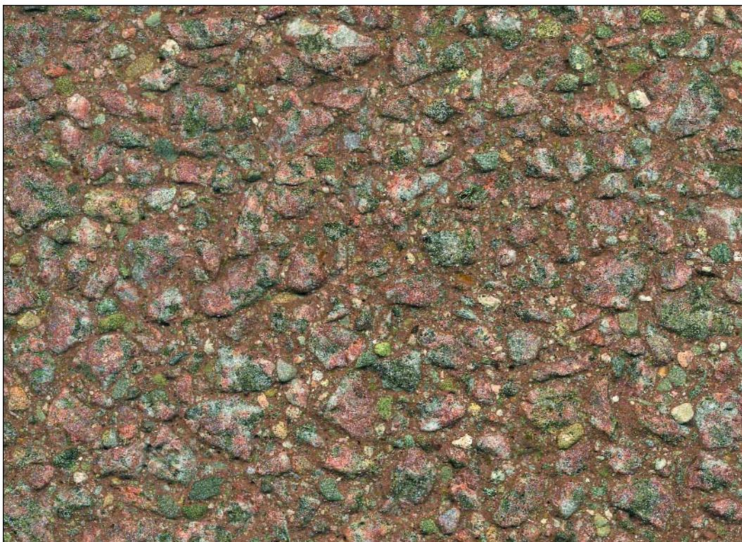
CPCI 174 red granite, natural concrete sand, grey cement, red pigment, heavy sandblast
