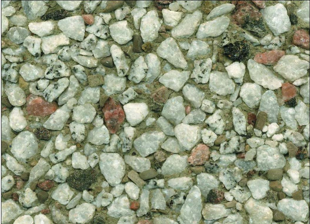
**CPCI 110** calcite, light grey granite, empire red granite, northern pink granite, concrete sand, grey cement, exposed aggregate
