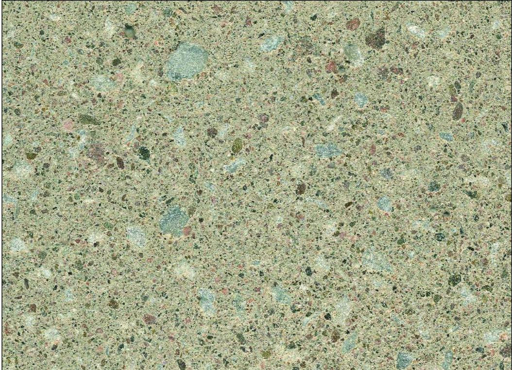
**CPCI 130** *Dufferin limestone, Ottawa red coarse sand, 70% white cement, 30% grey cement, medium sandblast*
