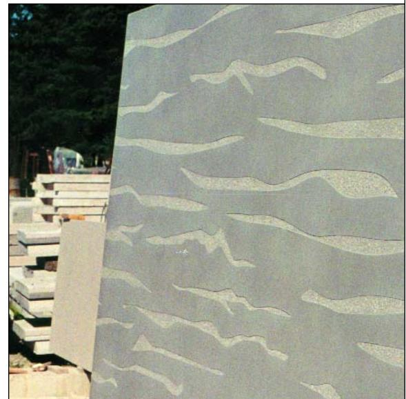
*Metal shield for sandblasting selected areas of a precast panel.*
