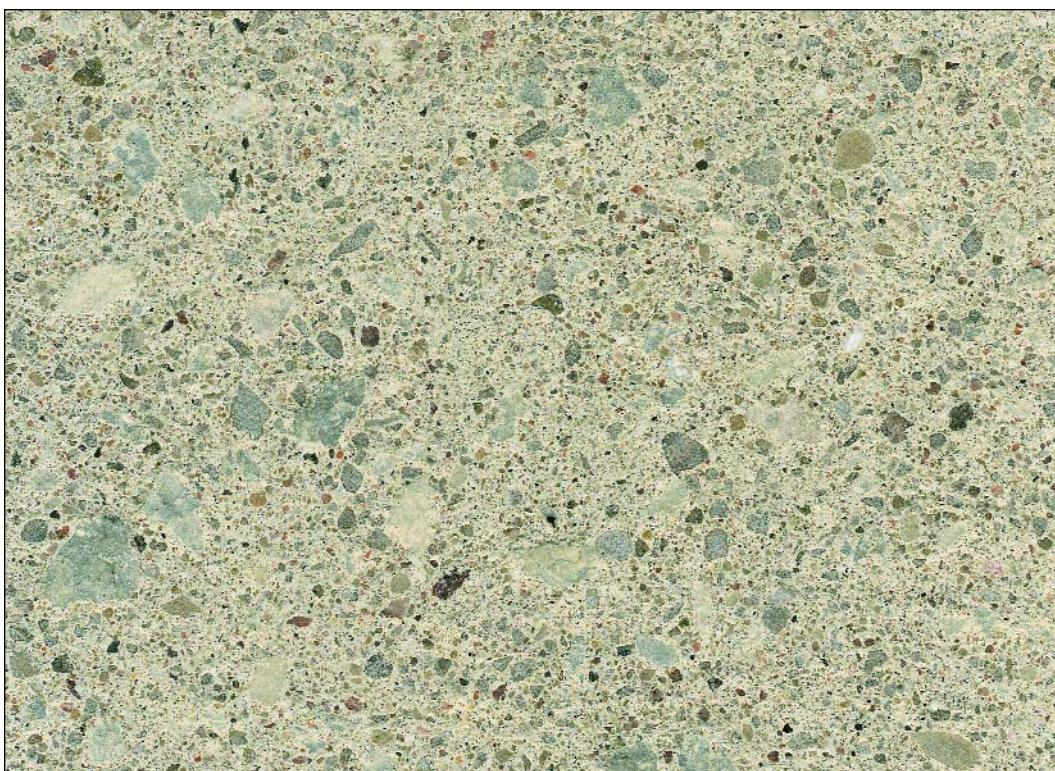
CPCI 150 *limestone, concrete sand, white cement, medium sandblast*
