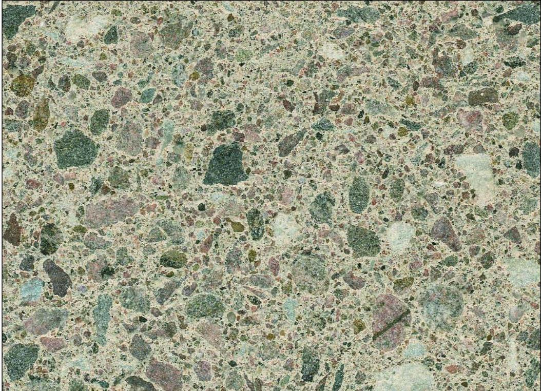
**CPCI 126** buff limestone, Ottawa red granite, Ottawa red coarse sand, white cement, heavy sandblast
