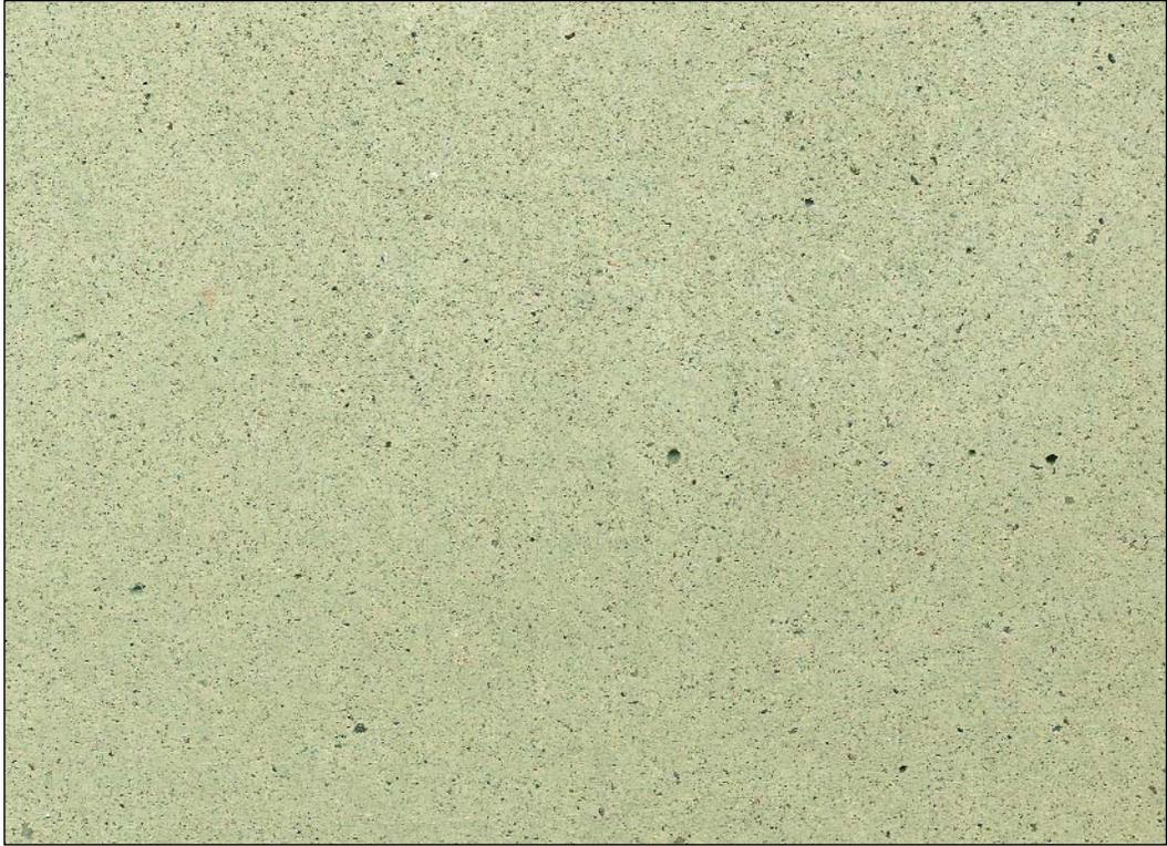
**CPCI 129** *Dufferin limestone, Ottawa red coarse sand, 70% white cement, 30% grey cement, light sandblast*
